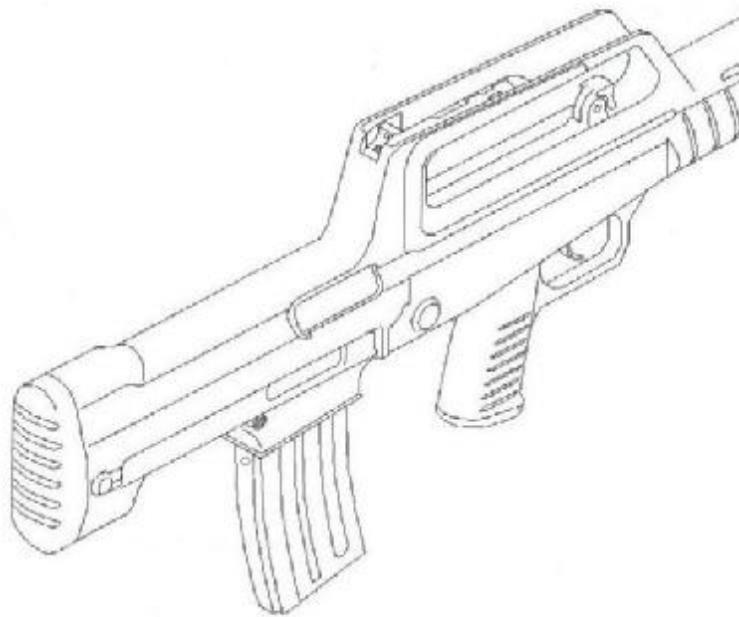
Fig. 8 Pull the bolt backward to feed a cartridge into the chamber
